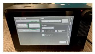
The camera will display a progress bar as it begins to perform a Black Calibration for each standard resolution and analog gain. This process will take approximately 10 minutes and display a completion message once finished.
