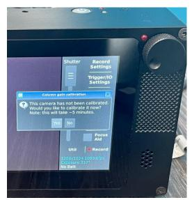
Wait for 15 minutes to let the camera and image sensor reach their operating temperatures, then press Yes. This procedure can be redone at any time via the Util -> Factory screen.
