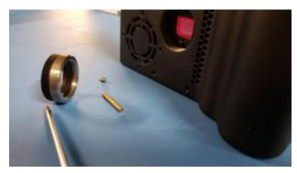
**2.** Loosen the two IR frame screws and carefully remove the frame without scratching the filter. Note that the filter is extremely sensitive and even the lightest touch can scratch it.
