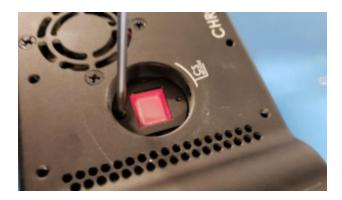
**3.** Using tweezers, very, very carefully push the IR filter up so you can grab one end. When grabbing it with tweezers, it will scratch it, only touch the part where the lens rests on the frame, not where the sensor looks through.
